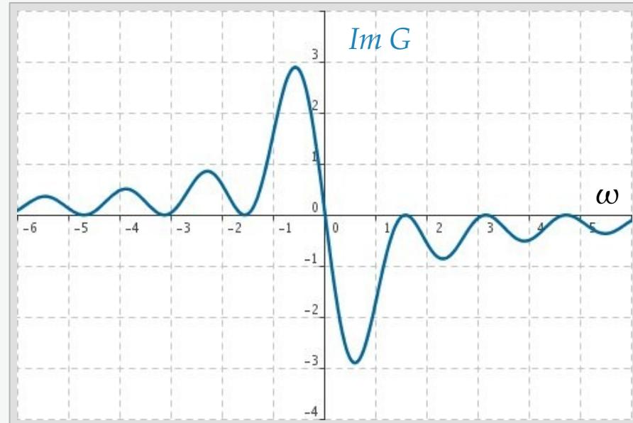
$$\text{Im}\{G(\omega)\} = -2 \frac{\sin^2(\omega T)}{\omega}$$
