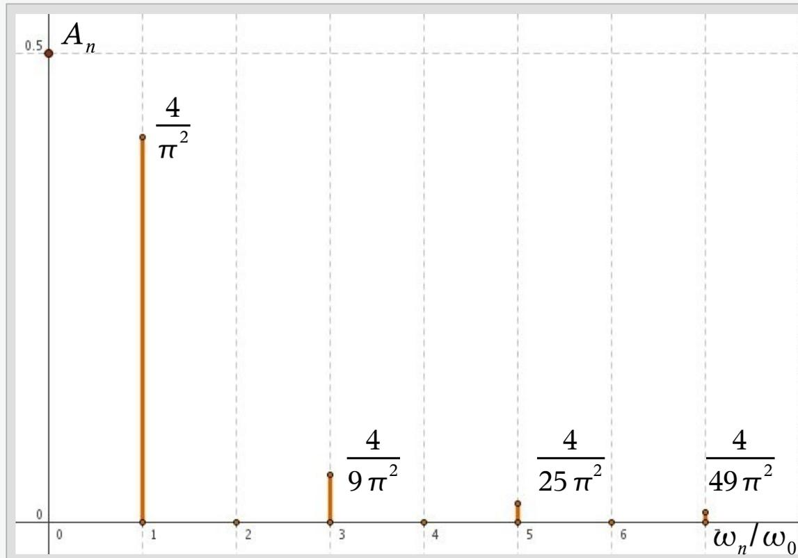
$$f(t) = \frac{1}{2} + \frac{4}{\pi^2} \left( \cos(\omega_0 t) + \frac{1}{3^2} \cos(3\omega_0 t) + \frac{1}{5^2} \cos(5\omega_0 t) + \dots \right)$$
